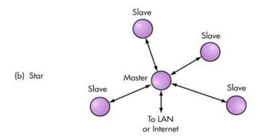
This configuration is commonly used where multiple distribution boxes are remotely connected to one common Internet connection. (Modem or Etherpad)
