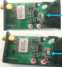
Switch the DIP switch to "Modem" for only one of the WL232s in the building the one that is in the same daizy-chain as the modem or etherpad
